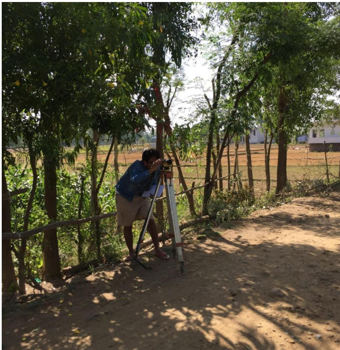
Fig: Measurement of cross-section through level machine
