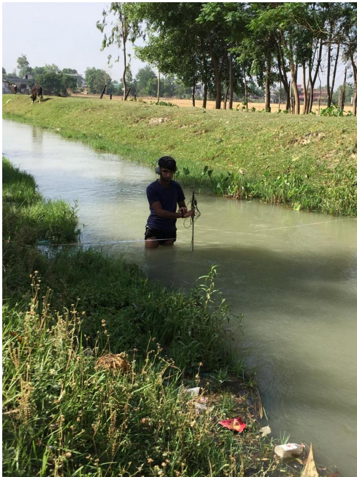
Fig: Flow Measurement of Sisaiya Branch
