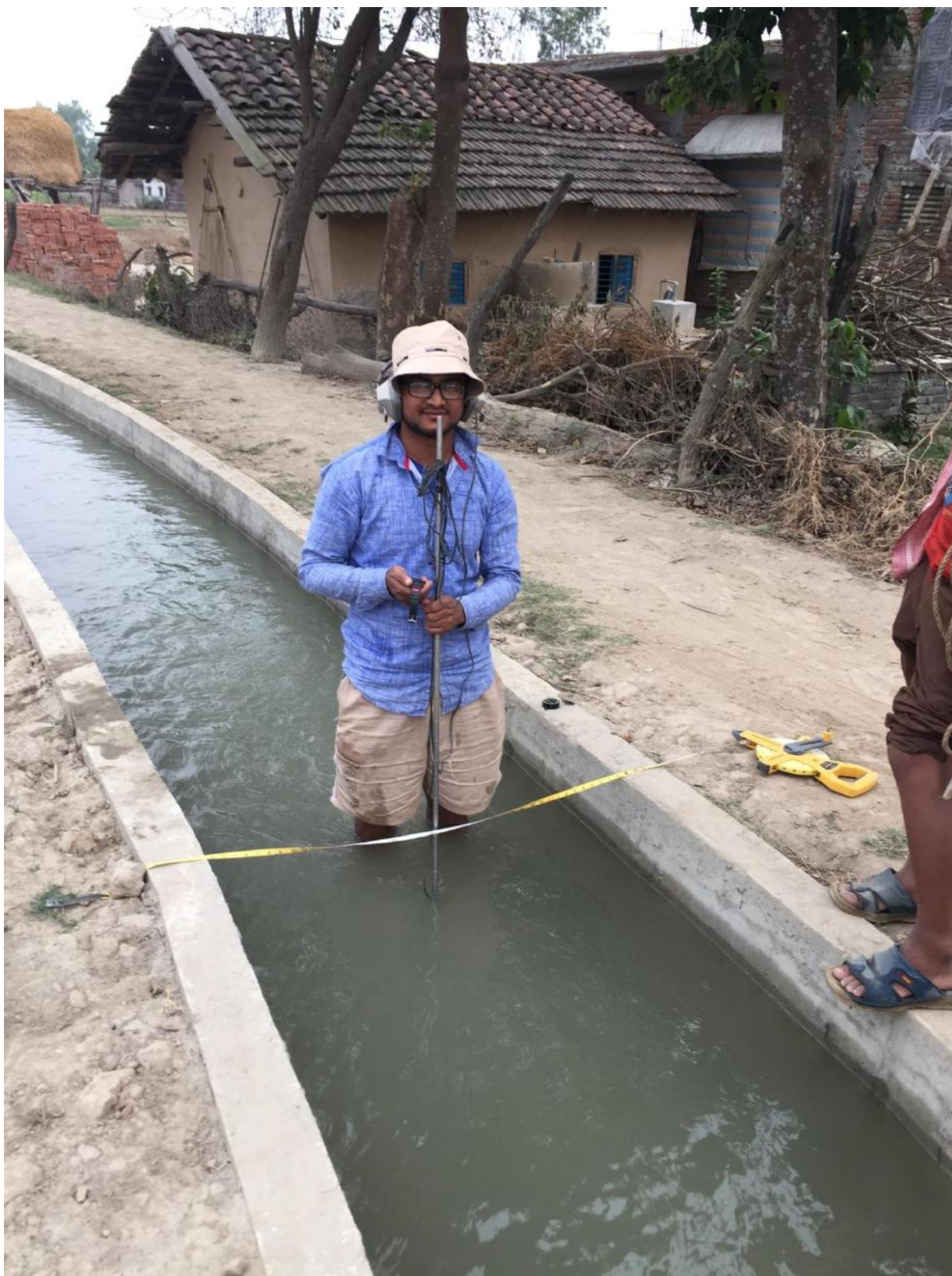
Fig: Flow Measurement of Imiliya Minor
