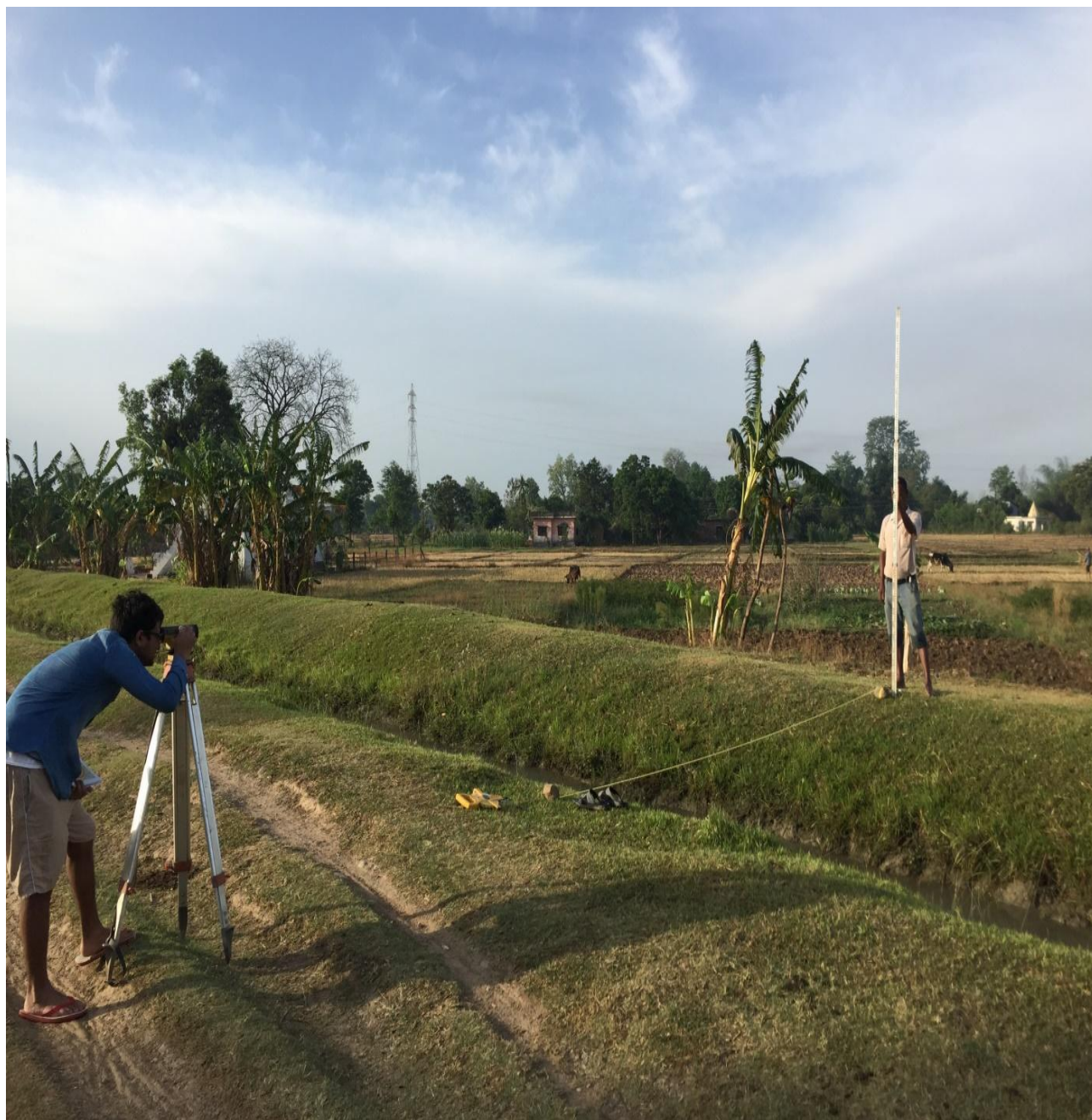
Fig: Cross-section Measurement of Daiji Minor
