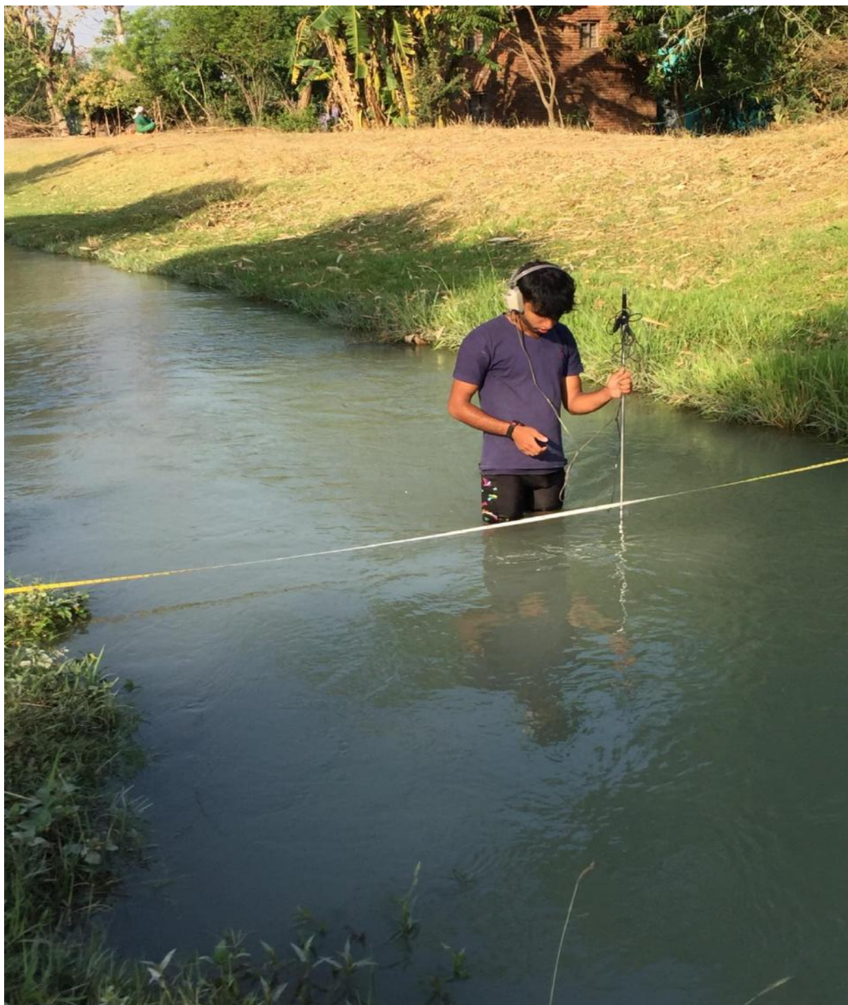
Fig: Flow Measurement of Majgaon Minor
