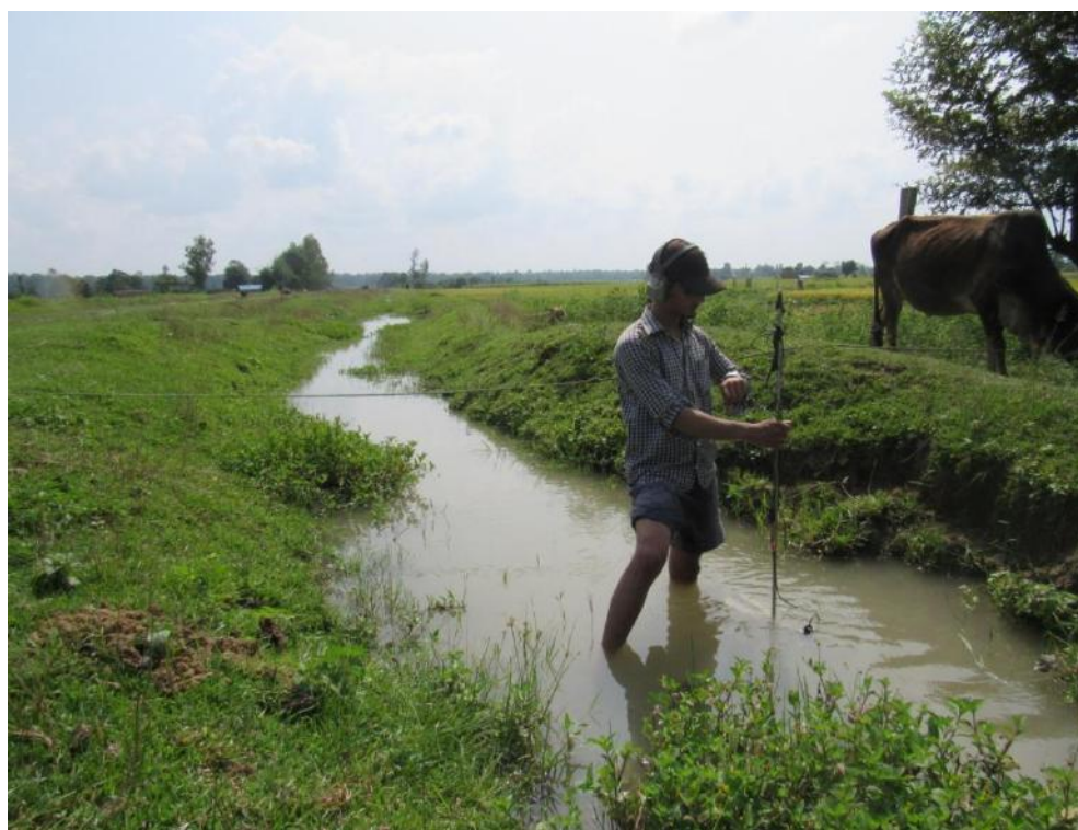
Fig: Flow Measurement of Salghar Minor
